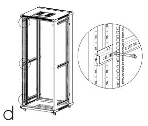
Grab the 19" rails (3) in the vertical and mount with 24 x bolt M6\*12 (B);
