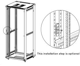
This installation step is optional. With 2 x bolt M5\*10 (A) fix this accessory to the frame;
