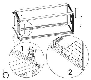
With the cable entry panel (9) and with the castors (10), assemble in the bottom plate with 24 x bolt M5\*10 (A);
