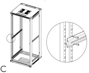
With the cabinet in the vertical, assemble the mounting angle (4) with 16 x bolt M6\*12 (B) in the horizontal sides of the cabinet;
