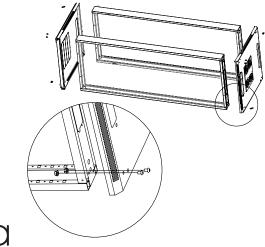
In this first step you will need the top cover (5), the bottom plate (8) and 2 x frame (6). Put the two parts of frame ready to assemble this part like picture with 16 x bolt M8\*12 (C) and 16 x flange nut M8 (D);
