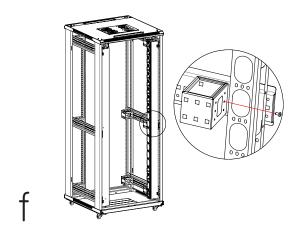
With 12 x bolt M5\*10 (A) fix the cable management (7) to the mounting spacer;
