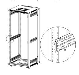
With the cabinet in the vertical, assemble the mounting angle (4) with 24 x bolt M6\*12 (B) in the horizontal sides of the cabinet;
