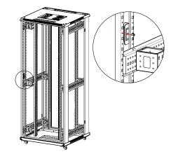
With 2 x bolt M5\*10 (A) fix the accessory to the frame;
