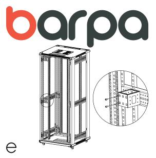
Grab the 19" rails in the vertical and mount with 24 x bolt M6\*12 (B);
