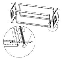
In this first step you will need the top cover (5), the bottom plate (10) and 2 x frame (6). Put the two parts of frame ready to assemble this part like picture with 16 x bolt M8\*12 (C) and 16 x flange nut M8 (D);
