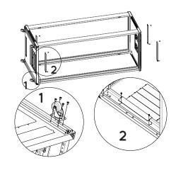
With the cable entry panel (11) and with the castors (12), assemble in the bottom plate with 24 x bolt M5\*10 (A);
