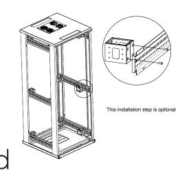
This installation step is optional. With  $24 \times bolt M6*12$  (B) fix the mounting spacer to the mounting angle;
