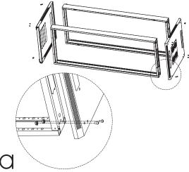
In this first step you will need the top cover (5), the bottom plate (8) and 2 x frame (6). Put the two parts of frame ready to assemble this part like picture with 16 x bolt M8\*12 (C) and 16 x flange nut M8 (D);
