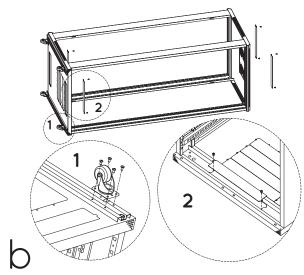
With the cable entry panel (9) and with the castors (10), assemble in the bottom plate with 24 x bolt M5\*10 (A);
