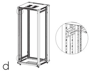
Grab the 19" rails (3) in the vertical and mount with 16 x bolt M6\*12 (B);
