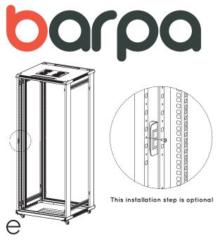
This installation step is optional. With 2 x bolt M5\*10 (A) fix this accessory to the frame;
