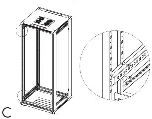
With the cabinet in the vertical, assemble the mounting angle (4) with 16 x bolt M6\*12 (B) in the horizontal sides of the cabinet;
